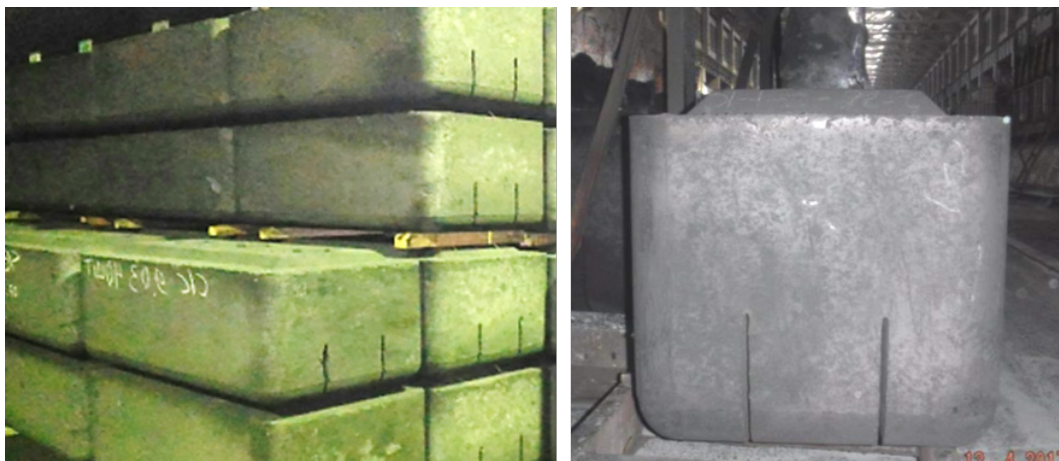
Figure 12. New optimized anode with chamfered edges.
