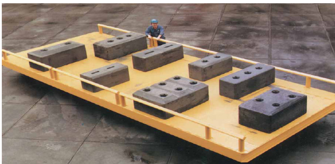
Figure 2. Prebaked anodes of various forms [2].
